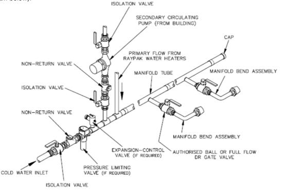
2. The **heating** water manifold (heating header assembly) must be designed to balance the flow from each unit i.e. each branch line must be the same diameter and length and be fitted with identical ball or gate valves (refer to diagram opposite).
