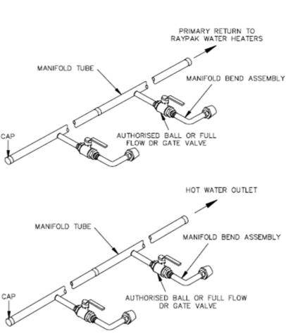
3. The **hot** water manifold (hot header assembly) must be designed to balance the flow from each unit i.e. each branch line must be the same diameter and length and be fitted with identical ball or gate valves (refer to diagram opposite).
