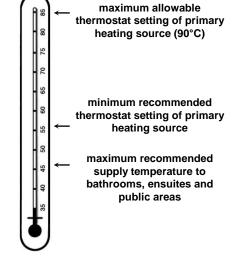
If this storage tank is installed as part of a solar water heater to an in-series continuous flow gas booster, then this requirement of AS 3498 can be satisfied provided the booster is energised, its preset outlet temperature setting is 70°C or higher and a remote temperature controller is not used.
