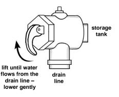
**Warning:** Failure to do this may result in the storage tank cylinder failing.
