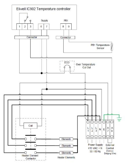
**Electric Heating Unit – Wiring Diagram**
