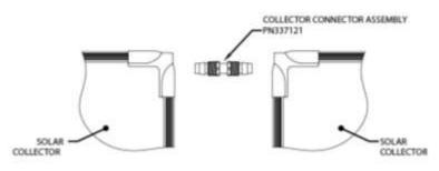
Detail 'B' Collector Connector Assembly (between collectors)
