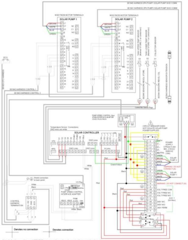
Note 1: A relay must be used if BMS/Aam connection voltage/current rating exceeds values shown. PART NO: 052547 WIRING DIAGRAM 3PH SOLAR PUMP SKID STANDARD REV AD
