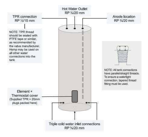
Note: Clearance around the water heater is required for servicing. (Typical clearances are: TPR valve removal 135mm, Element Cover and Element Removal 400 mm). Also, you must be able to read the information on the rating plate and if possible, leave headroom of one water heater length so the anode can be inspected or replaced.
