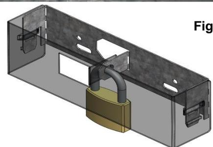
**N.B** Padlocks with a body wider than 30mm may not fit inside the body of the locking bracket
