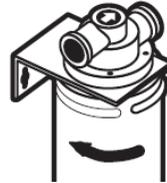
**Step 5:** Remove filter by lowering from housing. Ensure that minimal water is spilled within the boiling unit when removing the filter.
