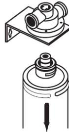
**Step 6:** Prepare new filter by removing the plastic wrap and taking off the top plastic cover covering the inlet to the filter.
