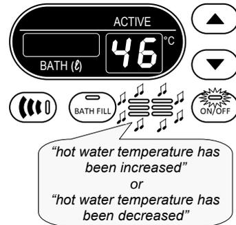
**During Step 6**, when the BATH FILL button is pressed to turn the Bath Fill mode on
