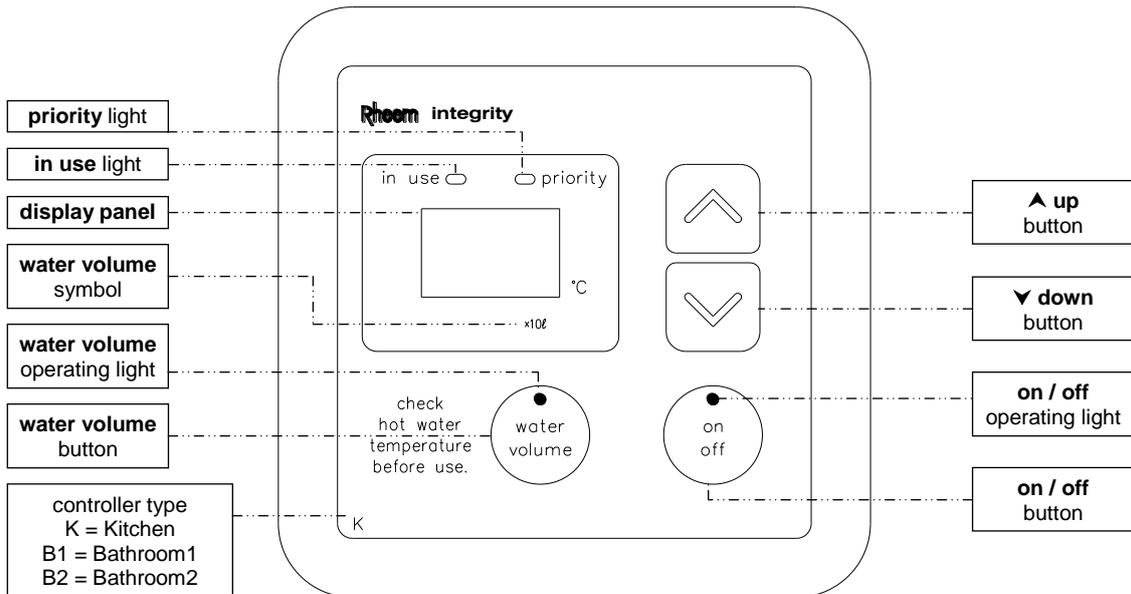
**Note:** **water volume** button, **water volume** operating light and **water volume** symbol are on the Kitchen controller only.
