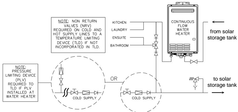
**Gas Booster for Closed Circuit Indirect Solar Preheater Installation
