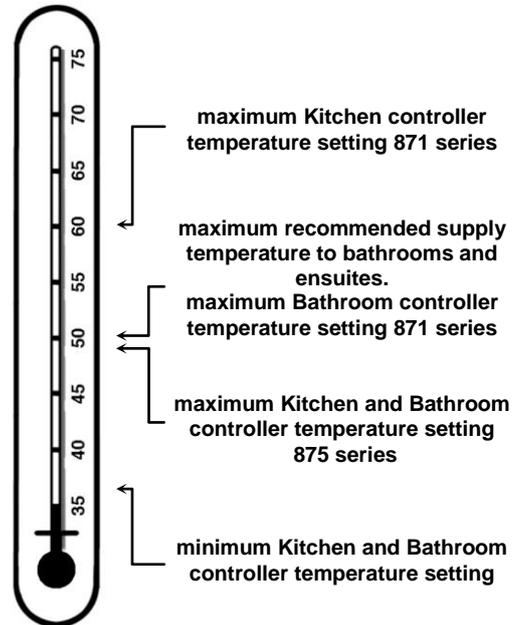
**Note:** For 871 series models manufactured before 2007, the factory preset outlet temperature setting is 50°C.
