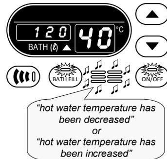
**During Step 9**, when the BATH FILL button is pressed to turn the Bath Fill mode off
