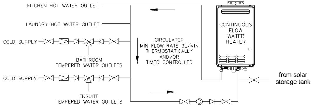
**NOTE:** A PLV IS REQUIRED TO BE INSTALLED ON THE COLD SUPPLY LINE TO THE TEMPERING VALVE IF A PLV IS INSTALLED ON THE COLD SUPPLY LINE TO THE WATER HEATER.
