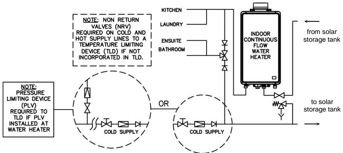
**In-series Gas Booster as part of a Closed Circuit Solar Water Heater Installation
