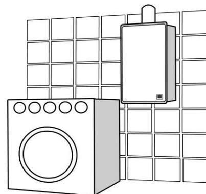
There are also special requirements in AS 5601 and AS/NZS 5601.1 for water heaters installed in a garage, an enclosed space and other locations. Remember all local authorities have regulations about putting water heaters into roof spaces.
