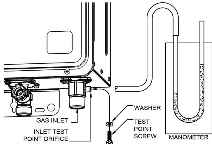
If the manometer reading is between the minimum and maximum inlet gas pressure ratings on the rating label, no adjustment is required.
