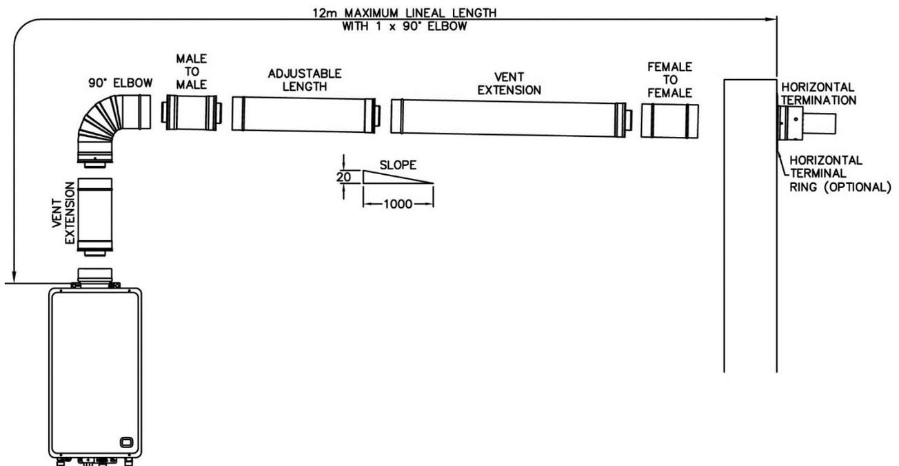
**Typical Installation – Horizontal Terminal with One Bend**
