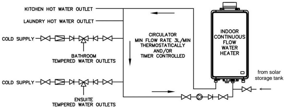
**NOTE:** A PLV IS REQUIRED TO BE INSTALLED ON THE COLD SUPPLY LINE TO THE TEMPERING VALVE IF A PLV IS INSTALLED ON THE COLD SUPPLY LINE TO THE WATER HEATER.
