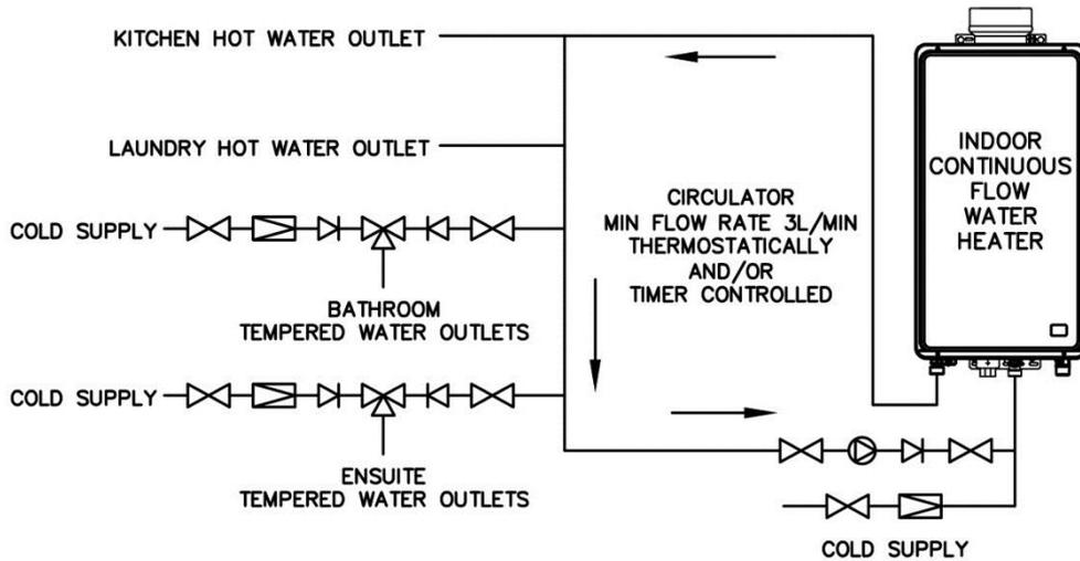
**NOTE:** A PLV IS REQUIRED TO BE INSTALLED ON THE COLD SUPPLY LINE TO THE TEMPERING VALVE IF A PLV IS INSTALLED ON THE COLD SUPPLY LINE TO THE WATER HEATER.
