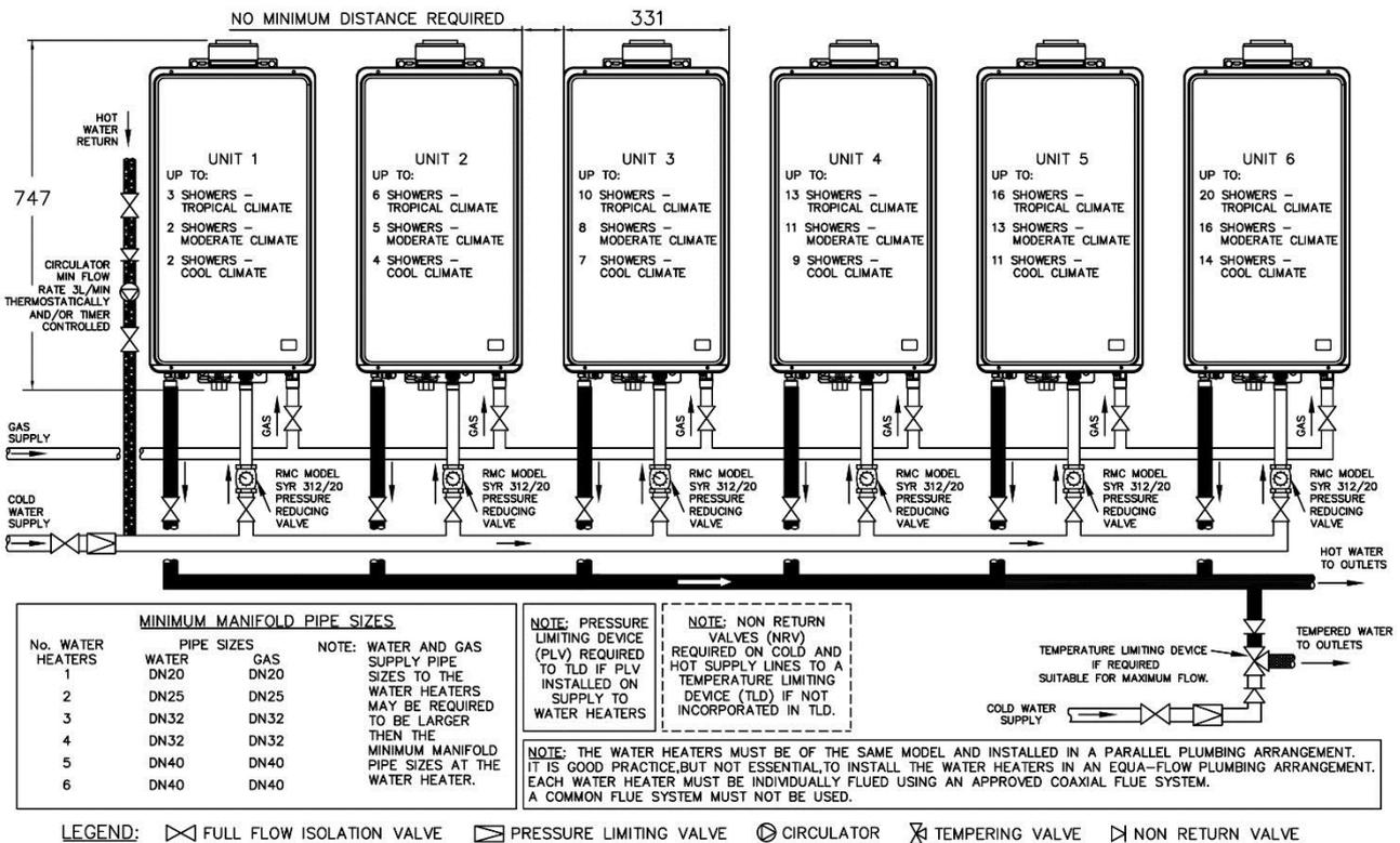
**Note:** An isolation valve and pressure limiting valve are not required on the solar preheat water line to the gas boosters as part of a solar water heater installation. A full flow isolation valve must still be installed on the inlet branch of each water heater.
