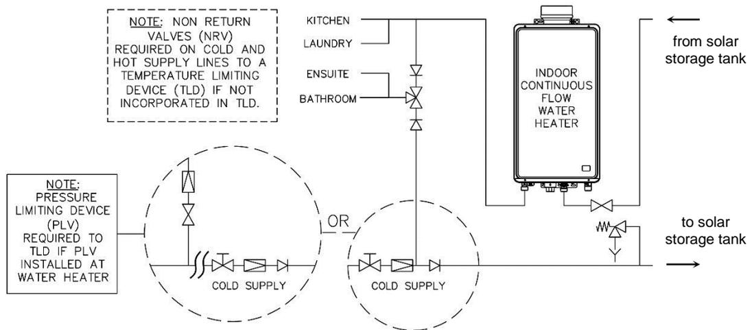
**In-series Gas Booster as part of an Open Circuit Solar Water Heater Installation
