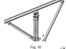
(4) Rotate the orientation of T head to fit the Tube Support to the post brace.
