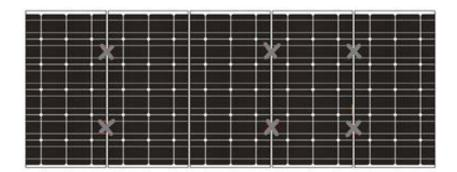
Install Grounding Clips at positions marked in diagram. Installation number of Grounding Clip = number of PV Module +1. Eg: 5+1=6 Grounding Clips image shown.
