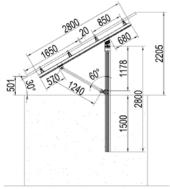
Side view drawings of support for 60 cell panels (up to 1700 x 1100 mm)
