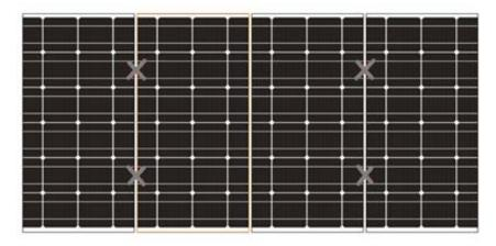
Install Grounding Clips at positions marked in diagram. Installation number of Grounding Clip = number of PV Module. Eg: 4 Grounding Clips in image shown.
