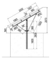
Side view drawings of support for 72 cell panels (up to 2000x1100mm)
