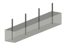
Apply Zinc Coating to upper section of C Post after ramming
