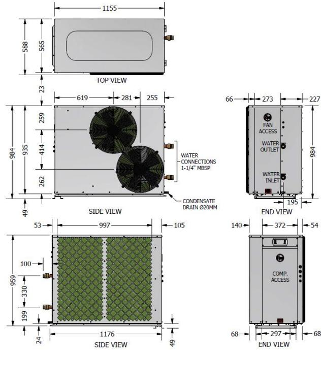
**RHEEM A2W 16kW- Ducted Horizontal Discharge 952016H0**
