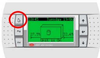
If the alarm light is flashing RED, check the alarm by pressing the alarm button. Phone your nearest Rheem Service Department or Accredited Service Agent (or Service Centre in NZ) to inform about the alarm.
